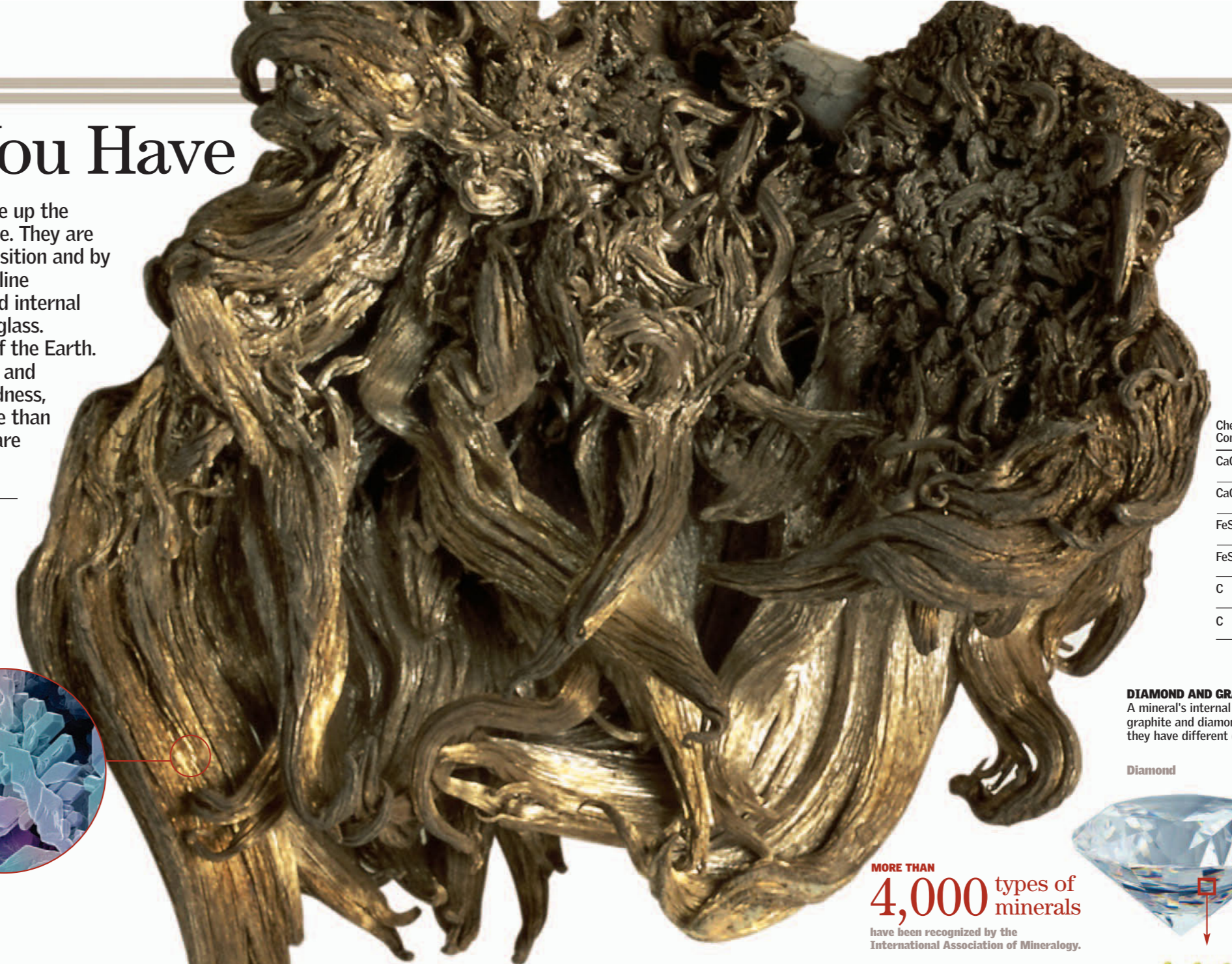
Microphotograph of silver crystal dendrites
