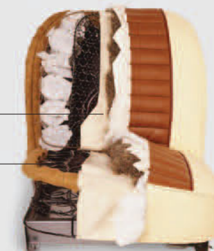
SEAT BACK Glass fiber SPRINGS Steel
