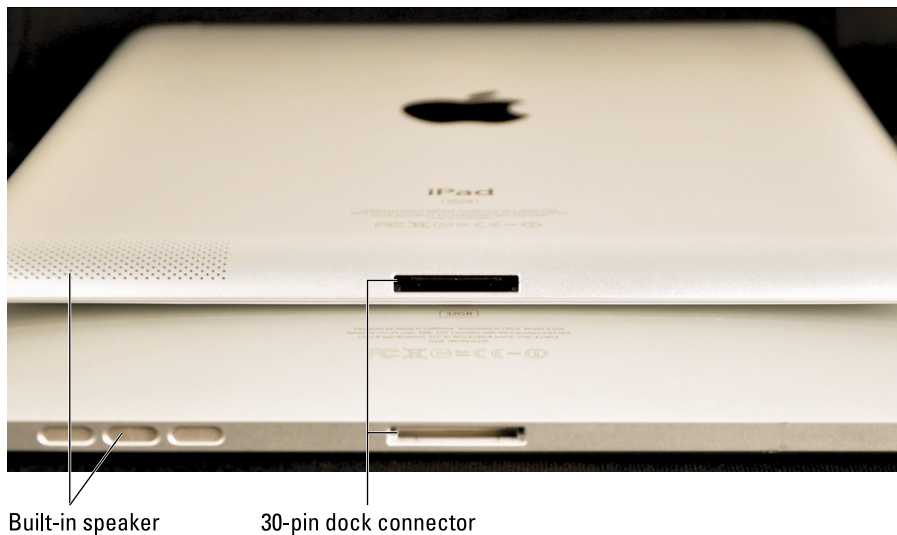
Figure 2-3: The bottom of the iPad and iPad 2.
