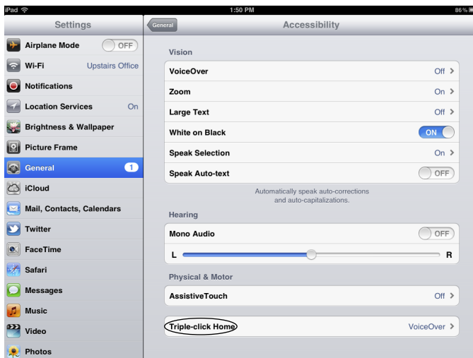
Figure 12-3: Triple-clicking Home can be set to quickly toggle core assistive features.
