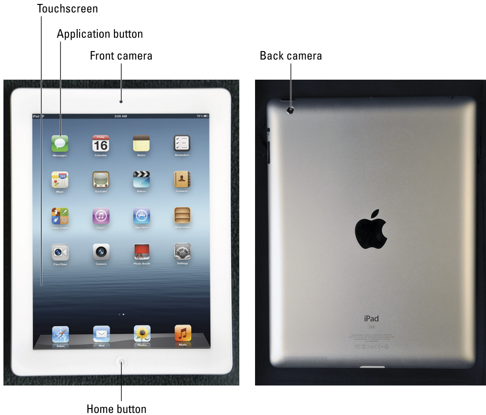
Figure 1-2: The iPad 2 and higher has an integrated microphone and camera.
