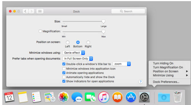
FIGURE 3-9: The Dock System Preferences pane (left) and the Dock Resizer shortcut menu (right).
