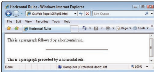
Figure 5-9: Use the <hr /> attributes to better control how a browser displays the rule.
