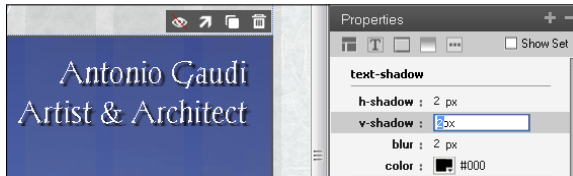
Figure 7-4: You can add drop shadows to images, <div> tags, and other elements using CSS3.
