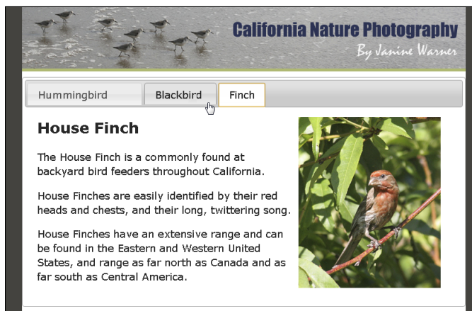
Figure 12-6: Tabbed panels enable you to change the content displayed on a web page when a visitor clicks a tab.
