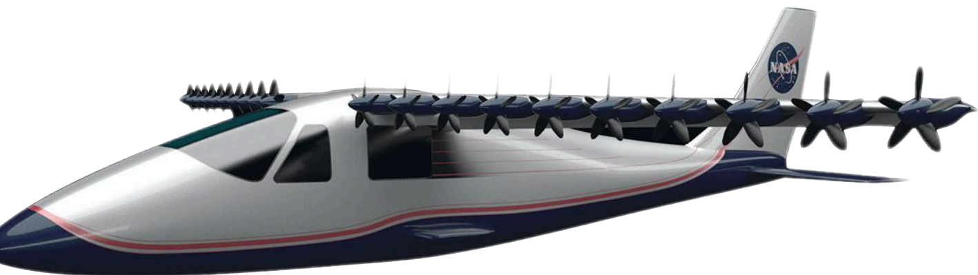
The Sceptor demonstrator design is based on a Tecnam P2006T light aircraft.
