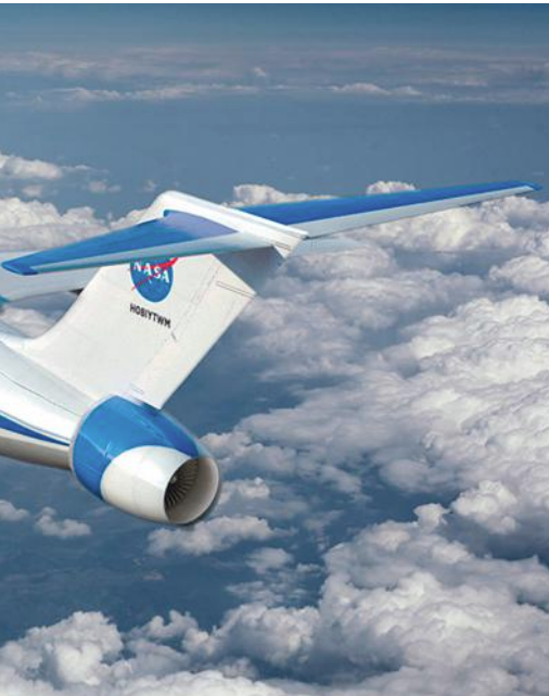
The Starc-ABL aircraft includes a proposed electric turbofan toward the rear of the aircraft.
