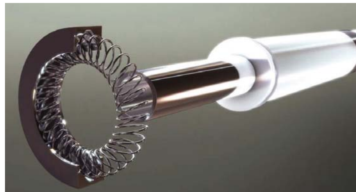
Here is a cutaway view of a canted coil-spring assembly that serves as an electrical contact. The male connector (shown) goes through the middle and makes contact with many of the spring's coils.
