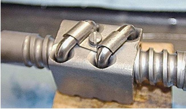
The Saginaw steering gear was a ball screw used on several automobiles in the 1950s and '60s. It features a dual-tube return that recirculates several ball bearings in separate circuits.
