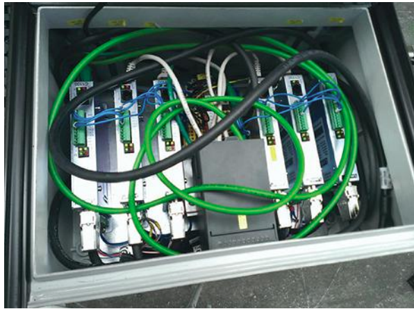
The linear motors are actuated by compact and lightweight servo controllers from LinMot that use ProfiNet interfaces.
