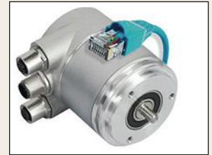
Using Ethernet-connected encoders, such as the Posital encoder above, provides connections between Industrial Ethernet and office Ethernet. This helps simplify the integration of production and management of parts by providing easier access.
