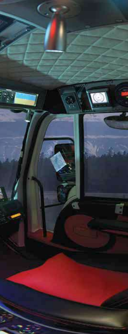
Left: In the cockpit, switches and screens over the windscreen control external sensors and lights, while the central console is for driving.
