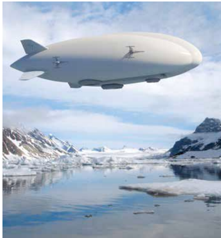
ABOVE: Lockheed Martin's Hybrid Airship can take off like a conventional airship, or like an aeroplane
