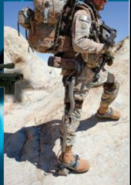
Above: The HULC allows humans to carry heavy loads across all terrains
