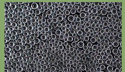
Droplets forming on a biphilic surface at -4°C
