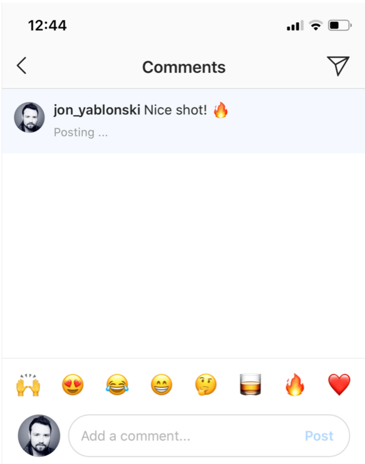
Figure 10-6. Instagram optimistically displays comments on photos before they are actually posted to improve perceived performance (source: Instagram, 2019)
