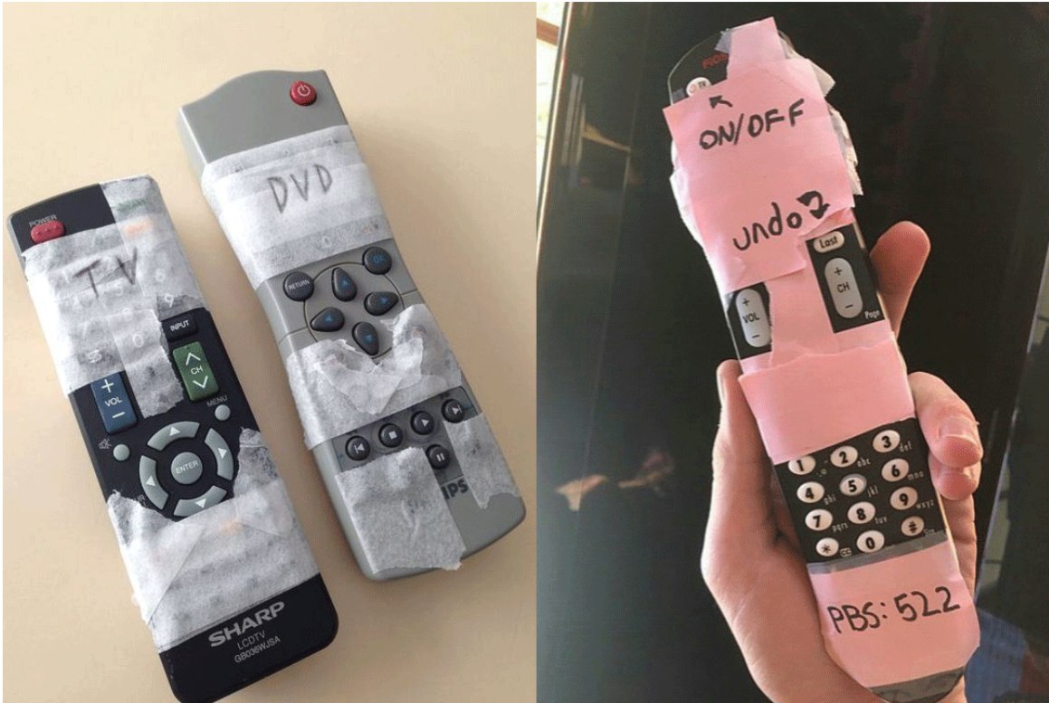
Figure 3-3. Modified TV remotes that simplify the “interface” (sources: Sam Weller via Twitter, 2015 [left]; Luke Hannon via Twitter, 2016 [right])
